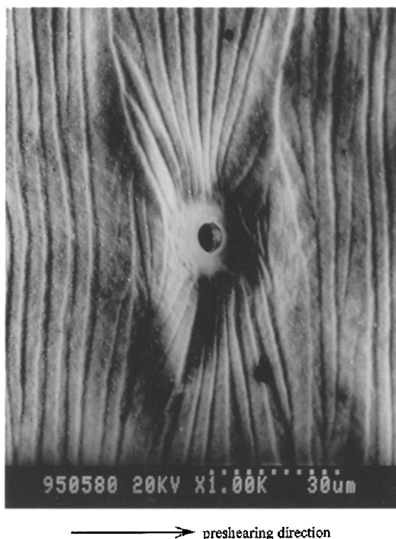
Figure 5. SEM micrograph of the presheared HPC film containing an air bubble.
